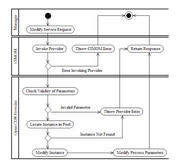
Fig. 4. UML activity diagram modeling a ModifyInstance operation. This operation involves three actors (the CIMOM, the OpenCDN provider and the management station). *Swimlanes* are used to group activities performed by the same actor.
