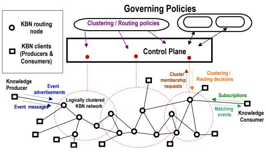
Figure 1: A control plane for a Knowledge Based Network
