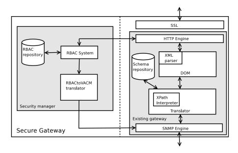
Fig. 1. Secure gateway functional architecture
