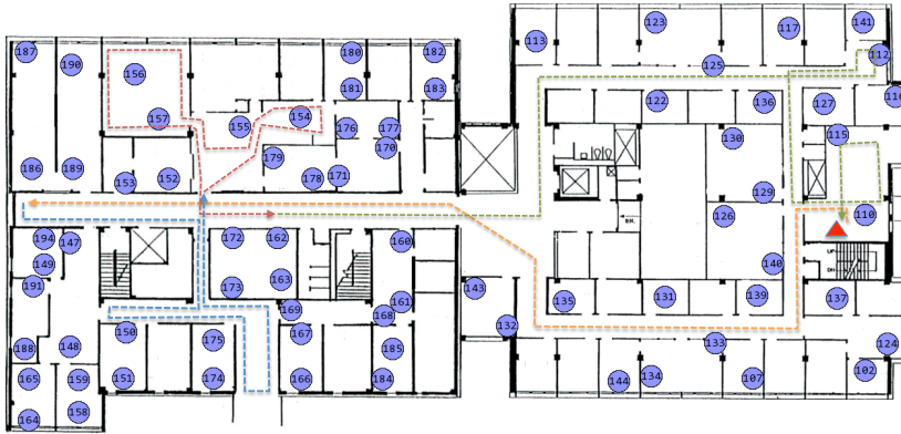
Fig. 6. A map of the WSN testbed at Washington University in St. Louis used in the medical patient monitoring application. The testbed nodes (circles) relay patient data to the monitoring station (triangle). The patient traverses the dotted lines.
