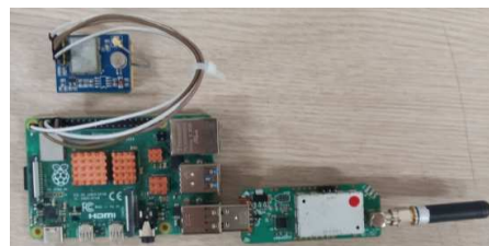
Fig. 2. HaLow Dongle attached to Raspberry Pi 4 with GPS
