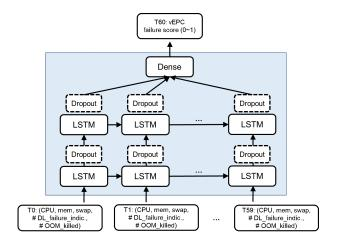
Fig. 4: LSTM model for predicting vEPC paging failure
