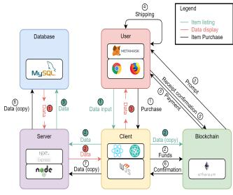
Fig. 4. E2E Trading Platform Architecture
