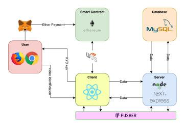
Fig. 3. KYC Platform Implementation Architecture
