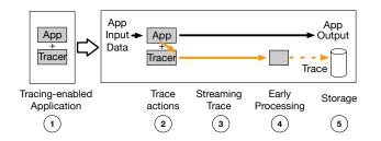
Fig. 2. Trace information flows through these stages: 1 an application is enabled for tracing (e.g., through recompilation or through OS services), 2 a trigger is stimulated by an input to take a tracing action, 3 trace information is emitted, then 4 this information might be lightly processed before it is stored 5. We reserve as much processing as possible to run offline.
