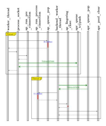
Fig. 4. We modified Apache to split worker threads into a front-half and back-half, with both halves communicating over a queue. This visualisation shows this new architecture. The value in green is the memory reference that is pushed onto the queue by worker\_thread and then popped by backend\_worker\_thread. This value is obtained from the traces, which had included extra information for simple memory tracing in this case.
