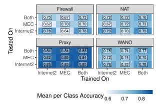
Fig. 6: Cross-prediction accuracy for different VNFs. Prediction horizon  $p=60\,s$ .
