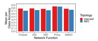
Fig. 4: Prediction performance w.r.t. different VNFs in the WAN and MEC scenarios. Prediction horizon p=60s.
