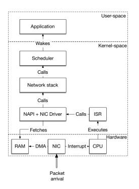
Figure 1. Schematic view of the path taken by a data packet – from Network Interface Card (NIC) to Application.
