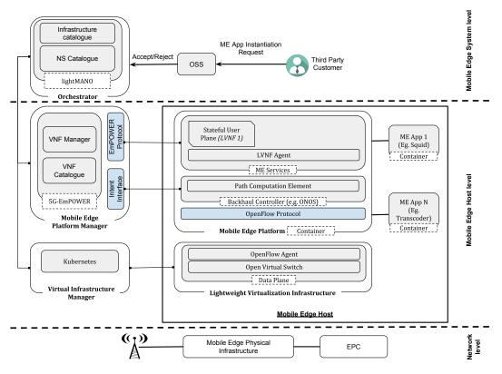
Fig. 3: lightMEC System Architecture.
