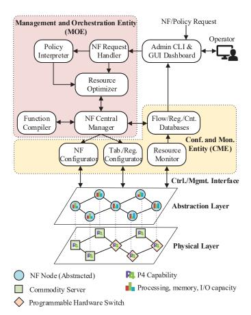
Fig. 1. Illustration of P4NFV architecture design. The physical layer consists of different P4-enabled entities which are abstracted in the abstraction layer for the ease of management.
