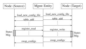
Fig. 5. The message exchange and states of NF (on/off) during migration with PR from an initial to a target NF node.
