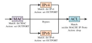
Fig. 4. Packet processing pipeline of a switch.
