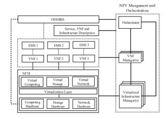
Fig. 2. ETSI NFV reference architecture framework [27]. P4NFV realizes the ETSI architecture, where in addition, physical resources are also P4-enabled.
