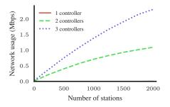
Fig. 6. Network usage for controller communication for an increasing amount of stations is very small.
