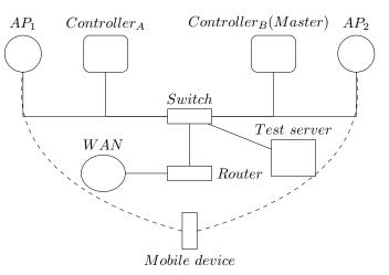
(a) DiMob test environment. The two nodes serve as the controllers.
