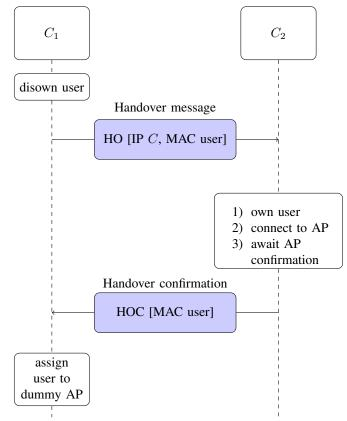
Fig. 1. The message flow for a foreign handover of a user.
