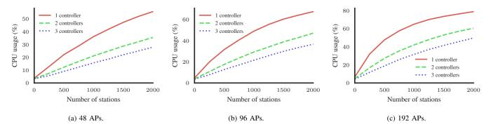
Fig. 4. CPU usage for an increasing amount of stations shows the benefit of multiple controllers in reducing load.
