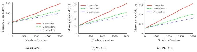
Fig. 5. Memory usage for an increasing amount of stations shows the benefit of multiple controllers in reducing memory.
