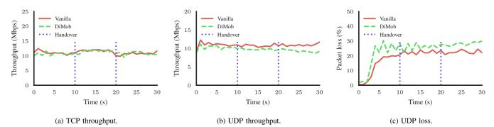
Fig. 3. Throughput and loss over time for UDP and TCP. Handovers (local for Vanilla and foreign for DiMob) at timestamps 10 s and 20 s are completely smooth.
