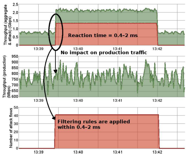
Fig. 6. Throughput and number of attack flows during the attack to NIIFI. Top: total volume of traffic (in green) and the volume flagged as attack (in red). Middle: production traffic that remains after filtering. Bottom: the number of detected attack flows. The attack has no visible impact to the production traffic because the reaction is much faster than the time resolution of the graphs.
