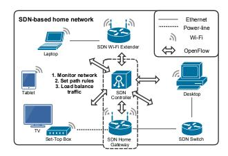
Fig. 1: SDN-based hybrid home network architecture.
