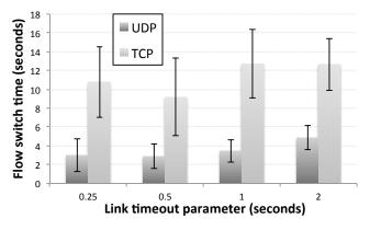
Fig. 5: Traffic downtime during link failure shown for both UDP and TCP traffic with changing link timeout values.
