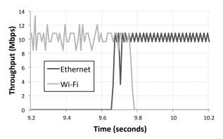
Fig. 3: Link switching with UDP traffic at 10 Mbps during normal conditions from Wi-Fi to Ethernet link.
