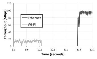
Fig. 4: Link switching from Wi-Fi to Ethernet link with TCP traffic during normal conditions.
