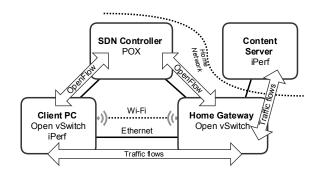
Fig. 2: Experimental set-up using SDN techniques.
