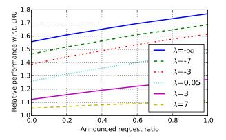
Figure 9. Impact of the session duration model parameter  $\lambda$  on the relative hit ratio compared to LRU with a deadline acceptance threshold  $\alpha = 25\%$  and deadline announcements 20-50 minutes in advance.
