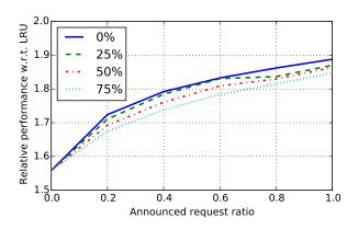
Figure 6. Impact of the deadline acceptance threshold  $\alpha$  on the relative hit ratio compared to LRU, when deadlines are announced 1h to 24h prior to playout.
