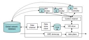
Fig. 3. Enhanced OpenFlow enabled switch structure.
