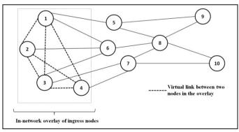
Figure 4. Example of a network and its associated full-mesh in-network overlay of ingress nodes
