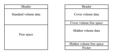
**Fig. 1.** The structure of a standard TrueCrypt volume (left) and one containing a hidden volume (right).
