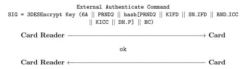
Step 8. Upon receiving 'OK', reader sends *Read Binary* Command in order to get the ICC's encrypted certificate plus MAC of encrypted certificate. However at this point, while card knows there is no man-in-the-middle because card checked the signature from reader, reader does not know whom he is talking to, and hence is unsure if there may be a man-in-the-middle attack, thats why he demanded the certificate.
